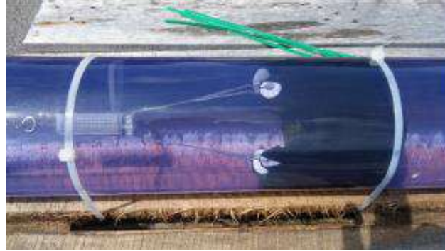
Parachute system with acoustic and optical (camera) sensor
